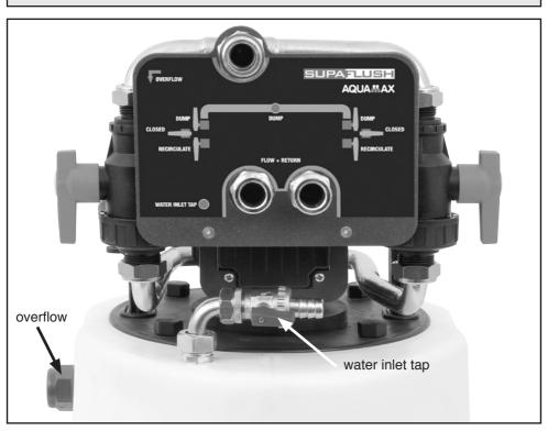
Using the female swivel fittings, screw the two lengths of hose provided to the "flow" and "return" 3/4" mi threads as clearly indicated in the centre at the base of the protection plate, fitted to the rear of the SUPAFLUSH pump.
